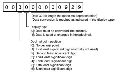
Since the display type is "0" in this case, the hexadecimal data is converted into decimal. 00000929H 2345
